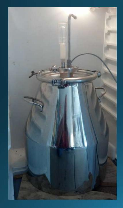
Jim Gress uses these hybrid stainless fermenters. They are 8gallon modified "milk-can" distilling kettles from Brewhaus.com that have been fitted with a Sanke Fermenter Conversion Kit from Brewershardware.com that features integrated thermowell, stainless racking cane and blowoff port. These can be pressurized to "push-rack" with CO2. The kettles are also available in a 15gallon size.
